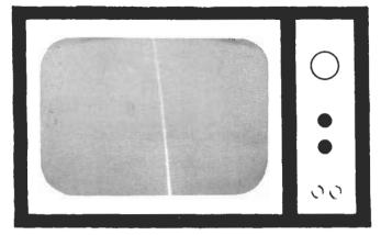
THE PICTURE illustrates what happened when a winding was open in the horizontal section of a deflection yoke. Since the line goes from top to bottom in the center of the screen, we know that high voltage and vertical height, both essential ingredients in obtaining a TV picture, are present. What is missing is horizontal sweep to spread the picture across the screen.
