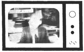
SOMETIMES when the brightness control is turned fully up, a picture may "bloom" or go out of focus. When the picture is out of focus all the time, no matter where the brightness control is set, suspect a defective picture tube, focus rectifier, or other component in the focus circuit. The first thing to do here is to locate the focus control on the rear apron and adjust for best focus. If that does not help, check for a defective component.
