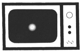
ERE IS a problem that usually crops up after you have performed some repairs on the chassis of a TV receiver. If you inspect the chassis, most likely you will find that you have forgotten to plug in the yoke assembly. This cannot occur on every TV chassis, because some have a low-voltage tie-in jack to prevent it from happening.
